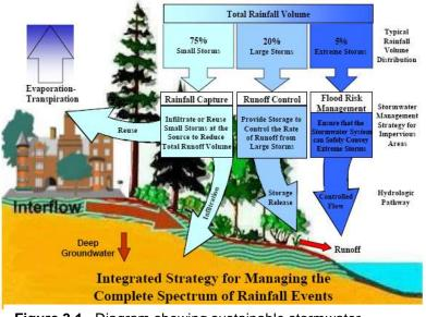
**Figure 3.1.** Diagram showing sustainable stormwater management practices. Source: Stormwater Planning – A Guidebook for British Columbia (BC Environment 2002).
